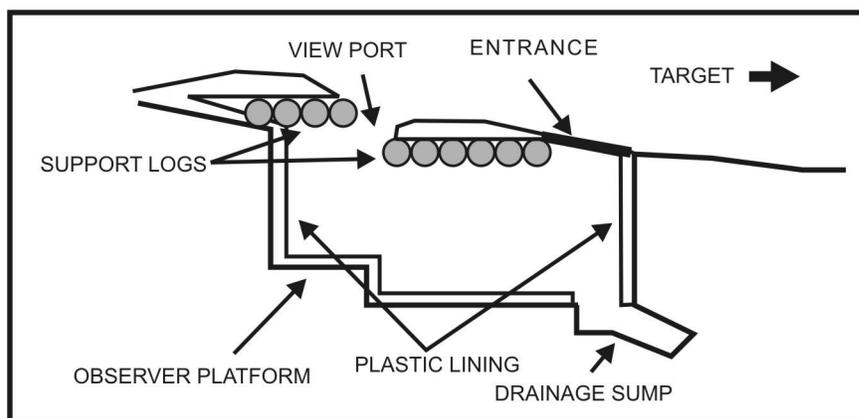
**Figure 5-31. Bunker-type underground observation post.**
